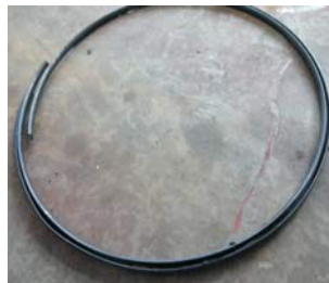
The C-ring was worn or broken.
