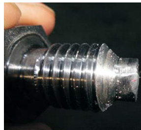
The end of guide pin was worn or the guide slot of the stem was deformed.
