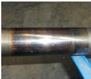
The stem part exposed to the packing was damaged as a result of strain.
