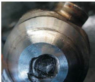
The sealing surface of the ball was damaged seriously.
