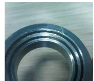
The sealing surface of the seat was scratched.
