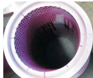
The periphery of the sleeve was subject to non-through type cracking.
